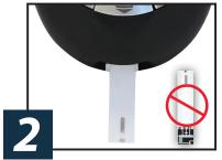
Remove Test Strip from vial and close vial immediately. Insert Test Strip into Test Port with Contact End (blocks facing up). The Meter turns on.
