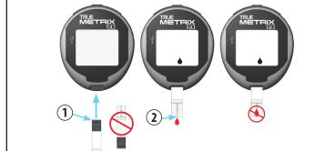
1. **Contact End** - Insert test strip into meter with contacts (blocks) facing up. **2. Sample Tip** - Touch Tip to top of drop of sample *after* Drop Symbol appears in the meter Display.
