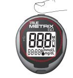
Start with the meter off. Press and hold the Set Button until the full Display appears and begins to blink. Release Set Button.
