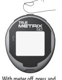
With meter off, press and release Set Button.
