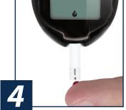
With Test Strip still in Meter, touch Sample Tip to top of blood drop and allow blood to be drawn into Test Strip. Remove from blood drop immediately after dashes appear across Meter Display.
